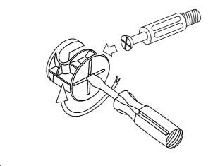
The head of the cam bolt goes into the open mouth of the cam nut. You then turn the cam nut so it tightens over the bolt.
