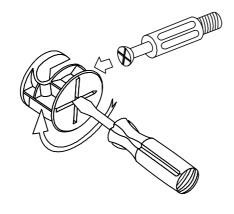
The head of the cam bolt goes into the open mouth of the cam nut. You then turn the cam nut so it tightens over the bolt.
